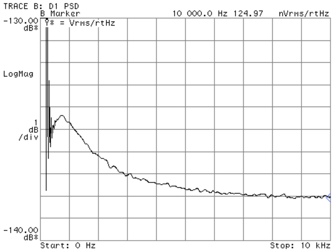
Figure 2.4: Output noise, DC-10 kHz with 12.5\Omega source resistance R_S , showing a 1/f corner at about 1.5 kHz.
