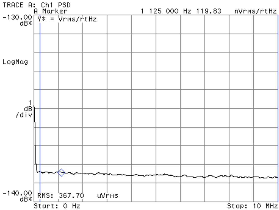
Figure 2.2: Output noise, DC-10 MHz with 12.5\Omega source resistance R_S ( -140 dBV = 1 nV input-referred noise; R_S adds 0.9 dB extra noise). Integrated noise of 368 \mu V in a bandwidth from 0.25 MHz– 10 MHz is 1.1 nV/ \sqrt{\text{Hz}} after source noise correction.
